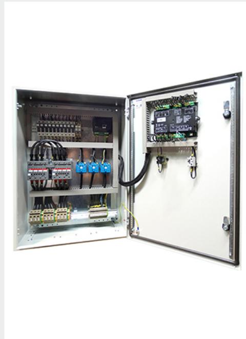
Cubicle composed of the electronic control module which is detecting a mains failure and of 2 contactors mechanically and electrically interlocked or a motorized switch controlled by the above electronic controller who are realizing the change of supply from the GEN SET or the MAINS to the load.
