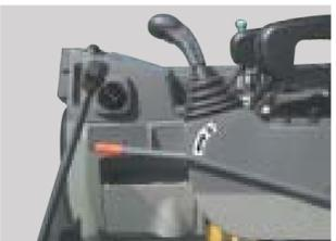
● **SAFETY LOCKOUT LEVER** for travel and slewing controls
