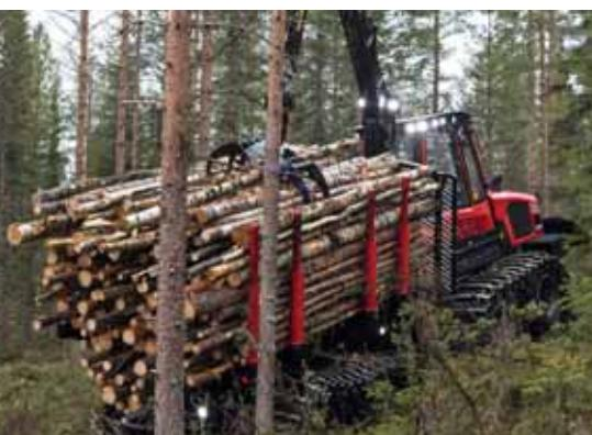
The crane has a long reach and a high net lifting force, a reliable pillar and hose routing solution and a Combi outer boom. Tiltable crane pillar (option) for efficient loading in steep terrain.
