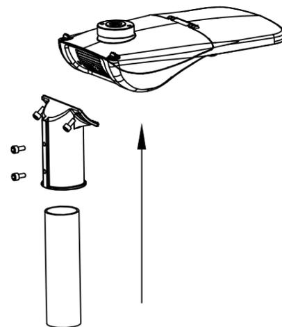
Fix the adaptor on the lamp body, sleeve the lamp pole into the adaptor and tighten it with screws.
