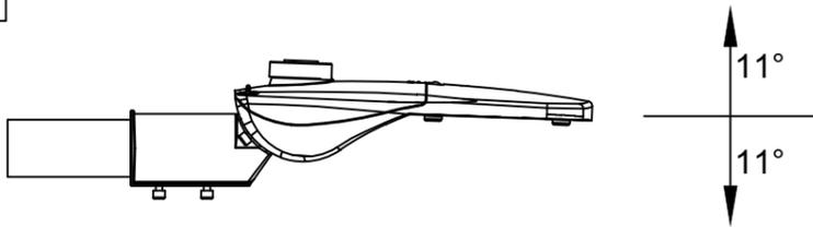
Loosen the M10 screw, adjust the desired Angle, and tighten the screw
