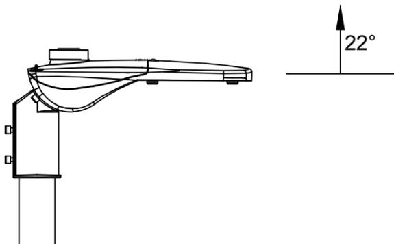
Loosen the M10 screw, adjust the desired Angle, and tighten the screw
