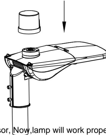
Install the light sensor, Now, lamp will work properly
