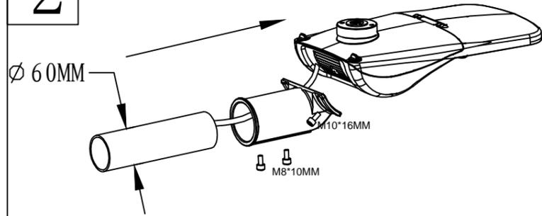
Fix the adaptor on the lamp body, sleeve the lamp pole into the adaptor and tighten it with screws.
