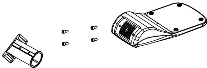
Open the box and take out the lamp body and lamp arm bracket, screws.
