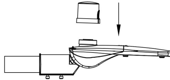
Install the light sensor, Now, lamp will work properly
