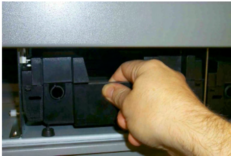
FIG 1-15 REMOVING A CASSETTE
