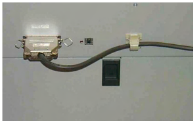
FIG 1-6 PARALLEL CONNECTION
