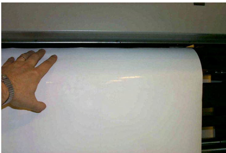
FIG 1-9 LOADING ROLL AT THE BACK OF DC3
