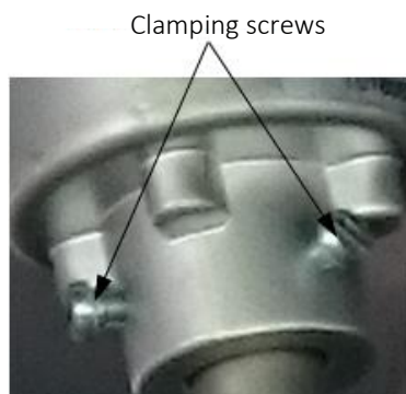
Illustration 196 Clamping screws
