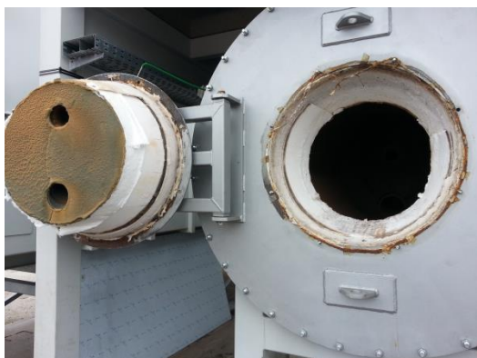
Illustration 189 Combustion chamber with door open
