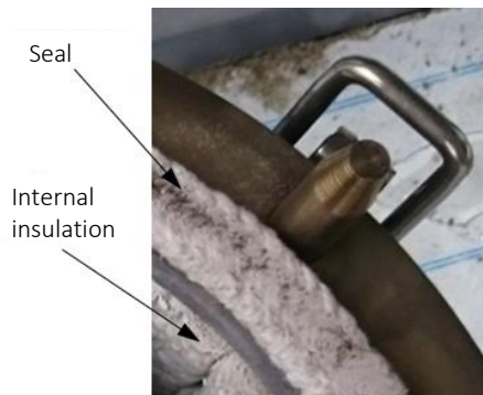
Illustration 218 HG cyclone slag pot insulation
