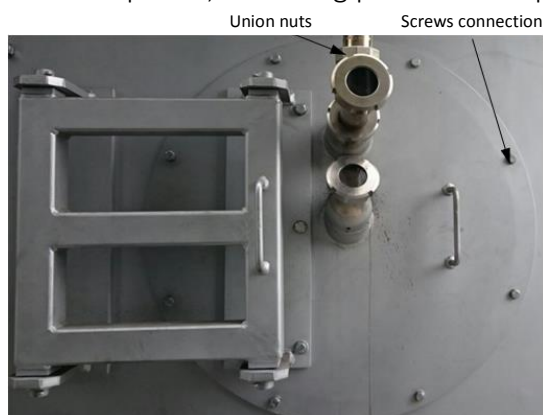
Illustration 188 Front side of combustion chamber
