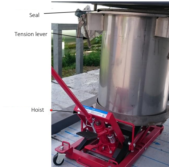
Illustration 213 Combustion chamber slag pot
