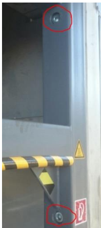
Illustration 230 Equipment container - Unit platform screw connection
