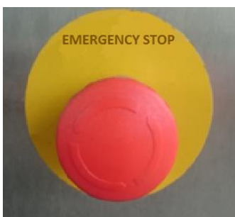
Illustration 25 Emergency Stop switch on the P500 unit
