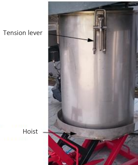
Illustration 217 Hot gas cyclone slag pot
