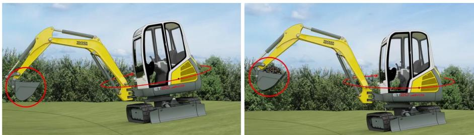
If the machine, specifically the swiveling axis, is at an angle, an additional torque demand is generated. Due to the VDS, a compensation of the revolving superstructure swiveling axis is possible in an exact vertical position.
