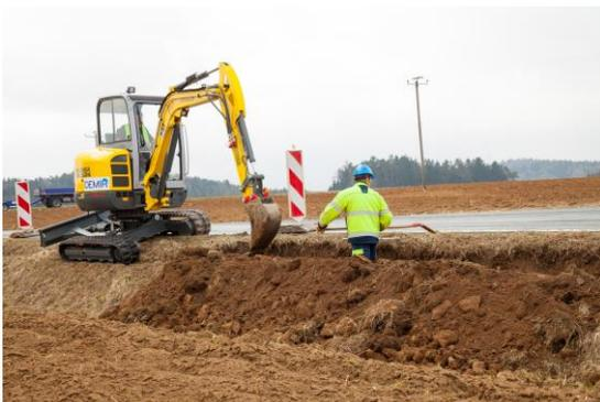
forward due to the uneven ground conditions will tip over much more easily forward than in the horizontal position. With VDS, the revolving superstructure is immediately brought into the horizontal position, which allows for considerably higher load carrying capacities and increases the stability by a considerable 20 percent when on a 15° gradient when fully extended. Whether handling a load hook on the backhoe bucket or with
