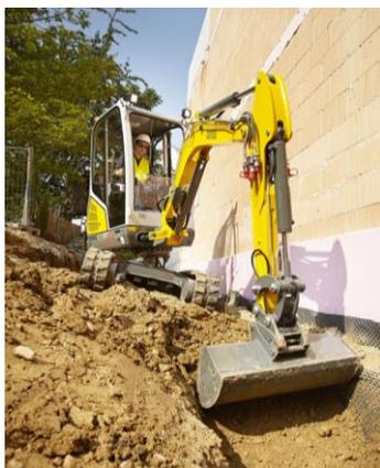
technology for compact excavators. Incorporating a maximum tilt of 15°, VDS compensates for the majority of slopes, slanted working surfaces, curbstone and sidewalk edges. VDS has a variable setting and the operator can easily activate it at any time via toggle switch in the cab.
