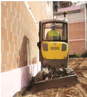
Despite the zero tail, the operator would have to work very carefully and therefore slowly without VDS so that the revolving superstructure does not hit the wall. Such work is accelerated considerably, thanks to the VDS technology.
