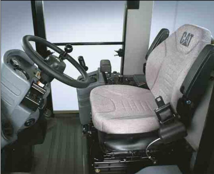
**Seat.** The comfortable and durable seat has adjustable fore/aft position, bottom cushion height, suspension stiffness and flip-up arm rests with a 76 mm wide retractable seat belt.
