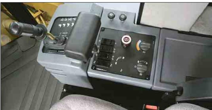
**Single lever control.** The single lever control for propel and vibratory On/Off provides simple and low effort operation. A padded adjustable wrist rest provides comfort.
