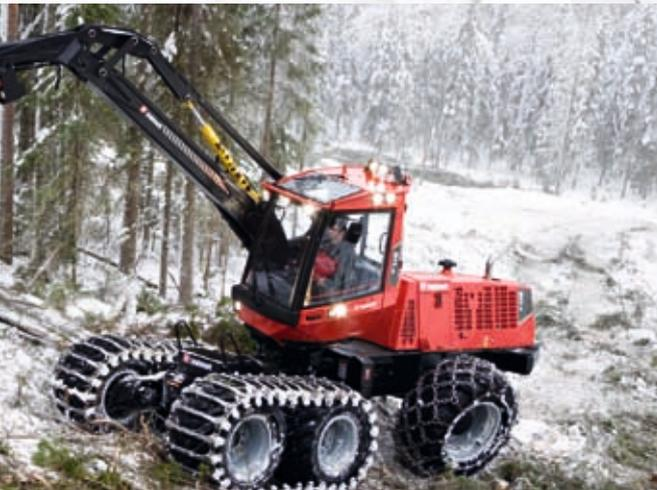
Stabilizer coupling and cab and boom leveling for optimum reach and stability
