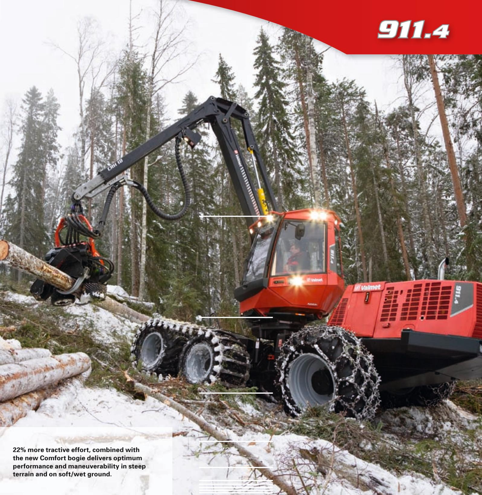
22% more tractive effort, combined with the new Comfort bogie delivers optimum performance and maneuverability in steep terrain and on soft/wet ground.
